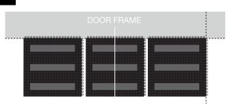
Unpack the tiles and allow them to acclimatise to the environment before you start installation. Mark the centre of the door frame (white line) and align the first tile with it. Lay tiles left and right of the first, until you cover the width of the space.
