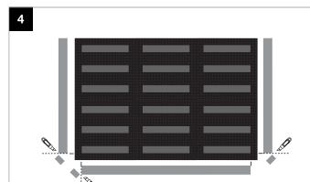
Having marked the aluminium profiles, cut off any excess with an appropriate tool e.g hack saw.
