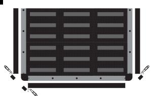
Use 5mm diameter flanged head screws to fix the aluminium profiles in place on all the sides. Once this is done the PVC corners can then be fitted into place.
