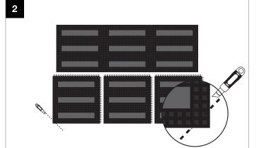
Use a dead blow hammer to join the tiles together. Once all the tiles have been connected, cut off a few centimeters of each corner tile at a 45° angle, this helps the corner profiles to fit.
