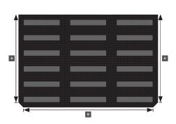
Measure 60mm from each corner to the door frame (A). Then measure 60mm from either corner across the front edge of the mat (B).
