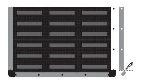
For a secure fitting, plot the drill points in the middle of the aluminium edges, and 300mm apart. The corners can only be fitted once the aluminium profile is screwed in to place.
